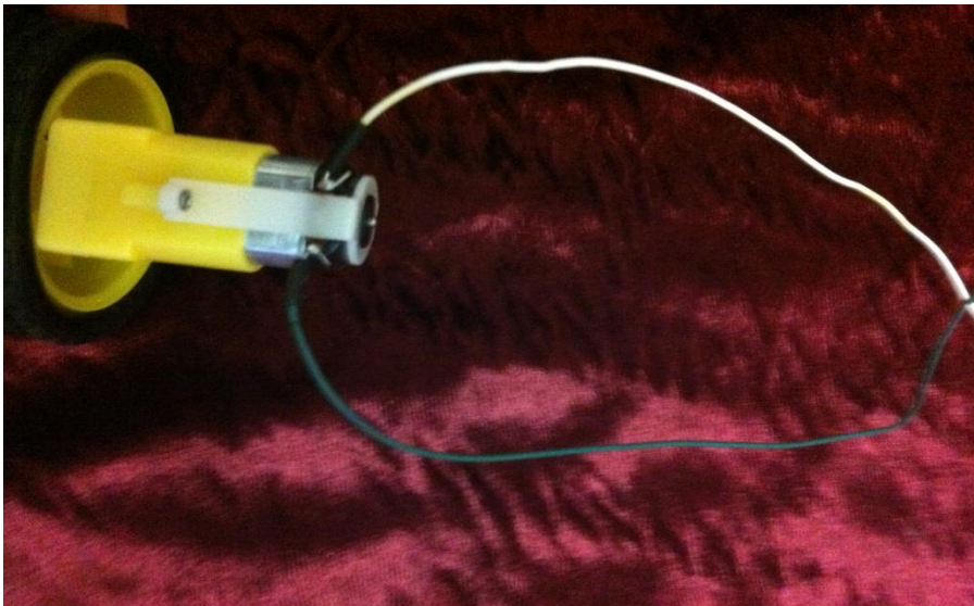
Figure 3-6 Soldering the wires with dc motor
