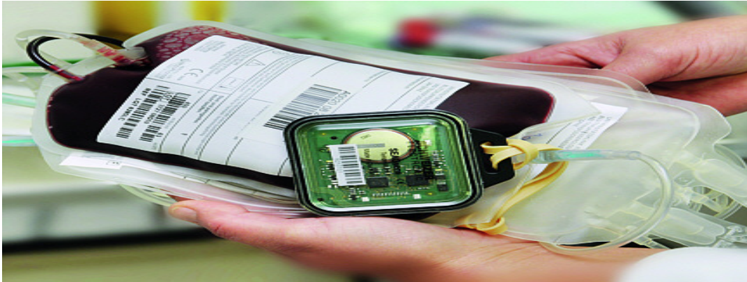
Figure 2.12 RFID Tag used in Blood Banks
