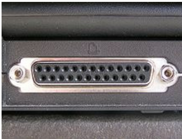
Figure 3.15 parallel port of a computer
