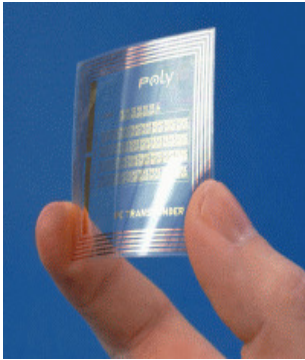
Figure 2.11 RFID tag can be used instead of the bar code in luggage
