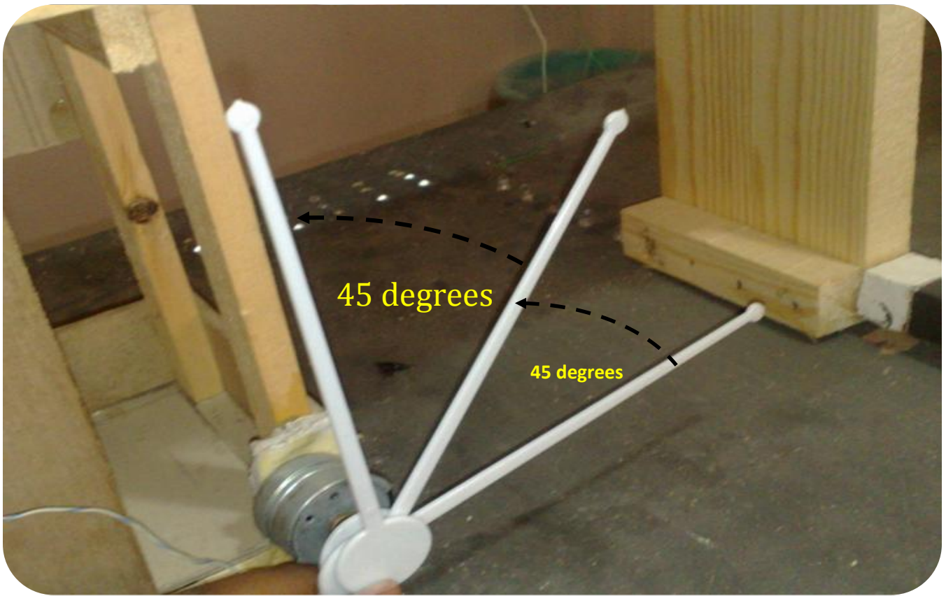
Figure 3.15: Stepper motor while opening gates. Opens using 45 degrees angles
