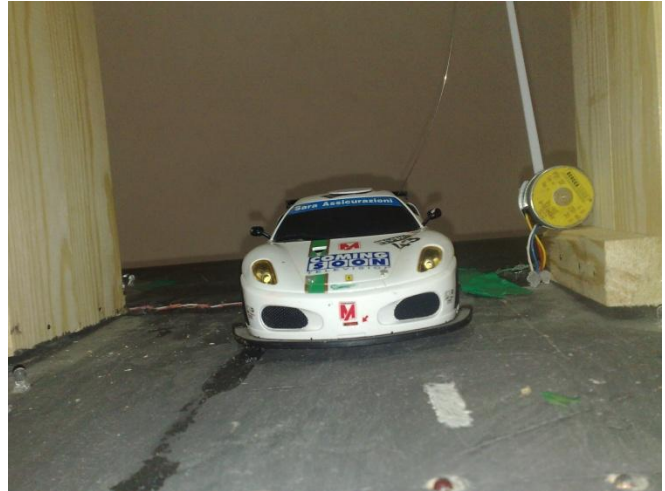
Figure 3.28: Gate is holding on cause car stop under it
