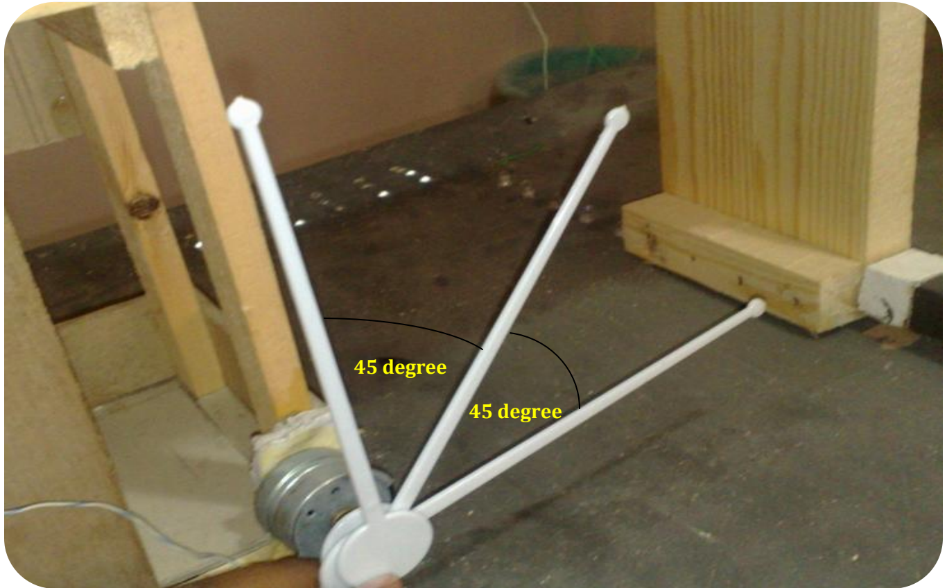
Figure 3. 18: Stepper motor while closing gates. Closes using 45 degrees angles
