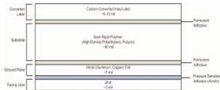
Fig. 1: Sample construction of the KU-Tag.
